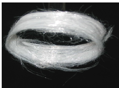
图 34 高强度 \text{ZrO}_2 连续纤维照片 Figure 34 Photograph of high strength \text{ZrO}_2 continuous fibers
